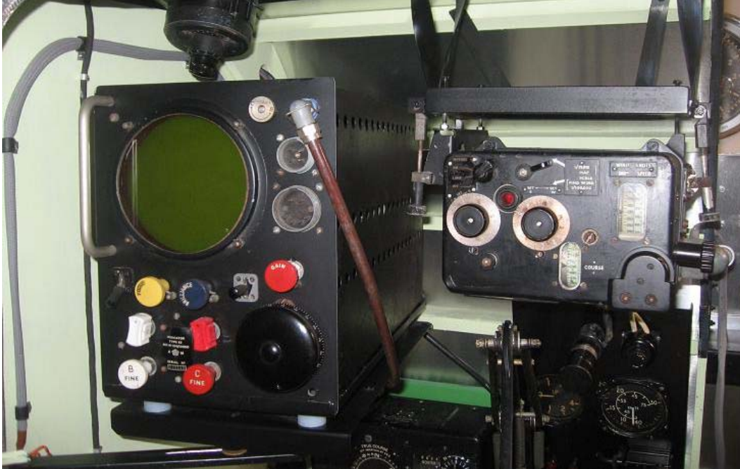
Figure 1: Mock-up of the black boxes used for radionavigation in an Avro Lancaster, one of the principal heavy bombers of the British Royal Air Force during the second half of World War II. The large circle on the left is an oscilloscope display that would show two wavy lines; using the knobs below to adjust the position of the wavy peaks would result in a pair of numbers. Photo from Peter Zijlstra, http://home.versatel.nl/gmwzijlstra-prummel/lancaster.htm .
